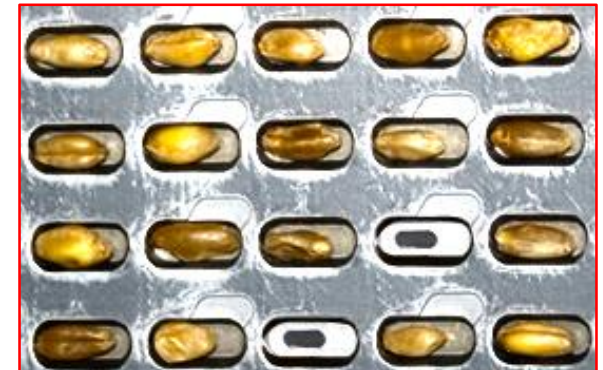
Inside cylinder, with detecting and blow opening
