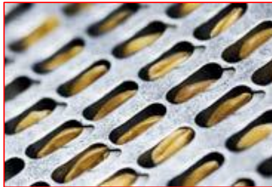
Inside cylinder, pockets filled with kernels
